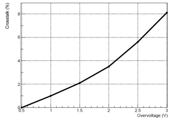
Fig.9 The optical crosstalk probability as a function of overvoltage
