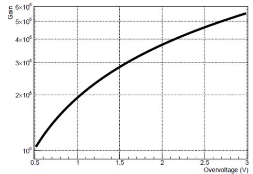
Fig.5 Gain as a function of overvoltage
