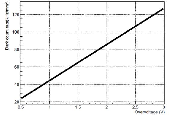
Fig.8 Dark count rate as a function of overvoltage
