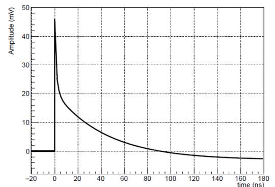
Fig.11 Typical signal of SiPM
