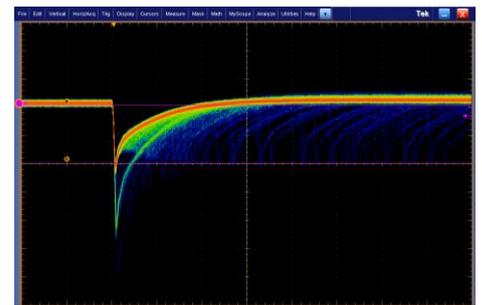
Fig.10 After pulse observed on oscilloscope (the blue pulse behind the main signal pulse is after pulse)
