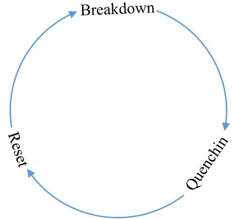
Fig.3 working process of single pixel
