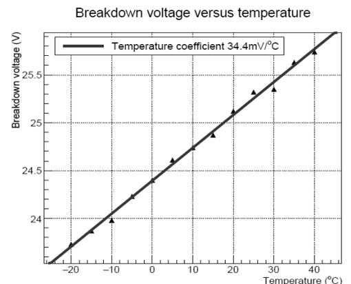
Fig.6 Breakdown voltage versus temperature
