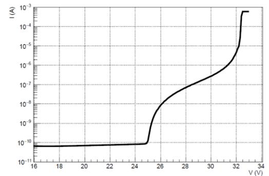
Fig.4 Typical I-V curve of SiPM
