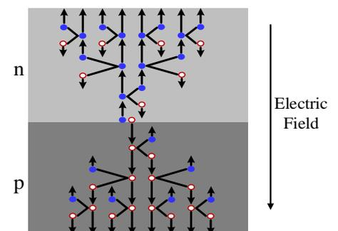
Fig.2 Principle of the avalanche multiplication process
