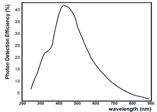
Fig.7 PDE as a function of wavelength
