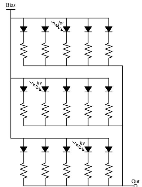
Fig.1 Schematic diagram of SiPM
