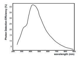
Fig.7 PDE as a function of wavelength
