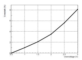
Fig.9 The optical crosstalk probability as a function of overvoltage
