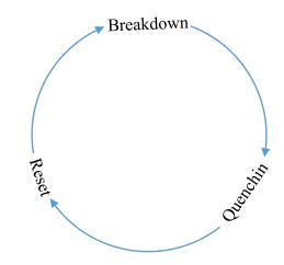
Fig.3 working process of single pixel
