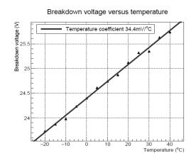
Fig.6 Breakdown voltage versus temperature
