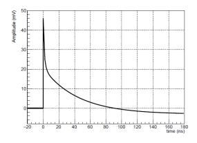
Fig.11 Typical signal of SiPM
