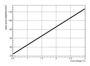
Fig.8 Dark count rate as a function of overvoltage
