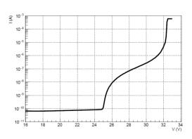
Fig.4 Typical I-V curve of SiPM
