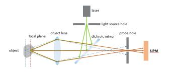
Application 3 Confocal Laser Scanning Microscope
