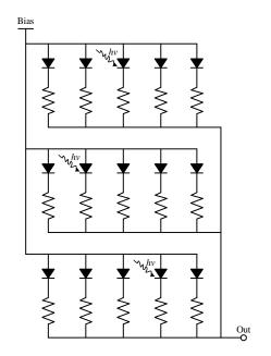
Fig.1 Schematic diagram of SiPM
