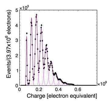
Figure 4. Response of the SiPM to a light source.
