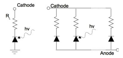
**Figure 3**. Structure of the single sensitive microcell (left) and schematics of the array of microcells composing the SiPM (right)
