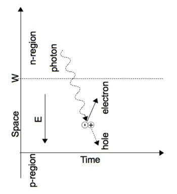
Figure 1. Principle of photon detection via photoelectric effect in a Silicon Detection Structure.
