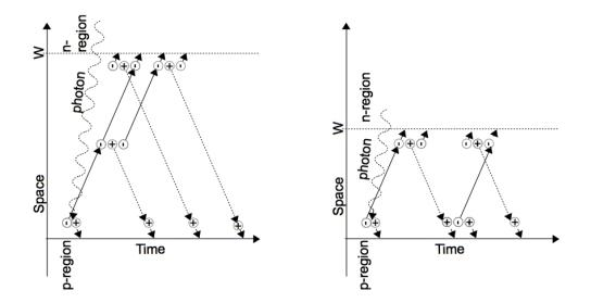
**Figure 2**. Two types of avalanche process in silicon detection structures. (Left) avalanche process carried by electron only; (Right) avalanche process carried by both electrons and holes.
